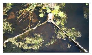
Figure 15. A small fyke net such as this one can be used to sample for juvenile fish as well as macroinvertebrates invertebrates. Larger versions are also available for sampling larger, adult fish. Photo courtesy of Doug Wilcox, US Geological Survey.
