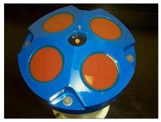
Figure 15. Image of a typical four-beam acoustic Doppler current profiler (ADCP) sensor head. The ADCP measures the speed and direction of ocean currents using the principle of "Doppler shift." Photo courtesy of NOAA Ocean Explorer.
