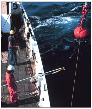
Figure 10. Retrieval of a current meter buoy. Photo courtesy of Commander John Bortniak, NOAA Corps. Publication of NOAA Central Library http://www.photolib.noaa.gov/corps/corp1716.htm
