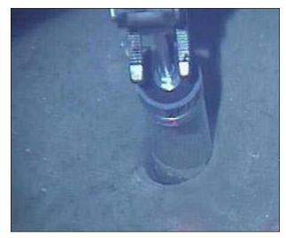
Figure 11. A push corer being inserted in the sediment using the manipulator arm of *Alvin*, a remotely operated vehicle (ROV) from Woods Hole Oceanographic Institution. Similar plastic tubes can be introduced manually in the sediment by diving or simply walking in an intertidal flat. Photo courtesy of NOAA Ocean Explorer.
