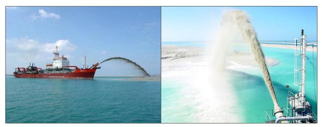
Figure 8. Dredgers throwing sand into a nourishment restoration project. Photo courtesy of Bert Visser's Directory of Dredgers. http://www.dredgers.nl
